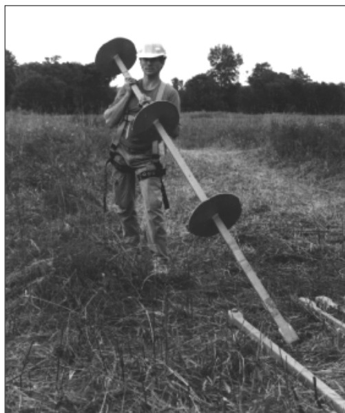
Photo 34. Tibor Latincics holding one-half of the Chance® six helix square shaft screw anchor. Photo courtesy of Mr. Tibor Latincics.
