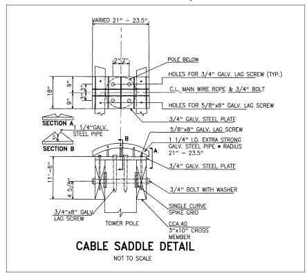
Figure 8. Cable saddle detail.
