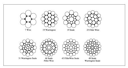
**Figure 12.** Strand patterns. *Courtesy of the Wire Rope Technical Board, Granbury, Texas.*
