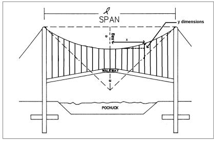
Figure 9. Nomenclature for wire rope equations.
