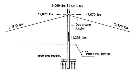
Ideal configuration: Departure angle for Catenary and Backstay cables are equal.
