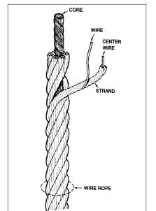
**Figure 11.** Typical wire rope components. *Courtesy of the Wire Rope Technical Board, Granbury, Texas.*
