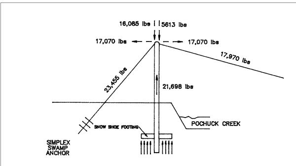
As-built Freebody Diagram. Departure Angle of Catenary and Backstay angles differ.
